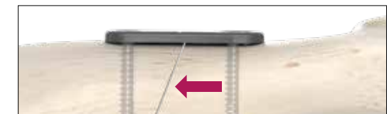
3. Additional 1.5mm of locking compression will occur as screw head engages into plate threads.
